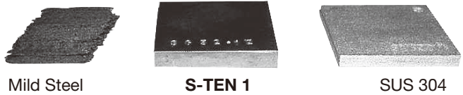
Photo 3.1 10.5% Hydrochloric Acid, 60°C, 72 Hrs
