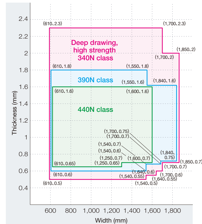
Deep drawing, high strength — 340N, 390N & 440N classes (base metal: cold-rolled coils)
